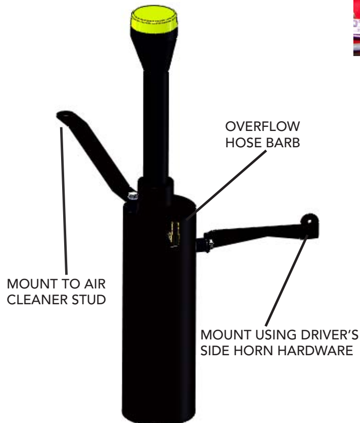
New Coolant Reservoir Mounted
