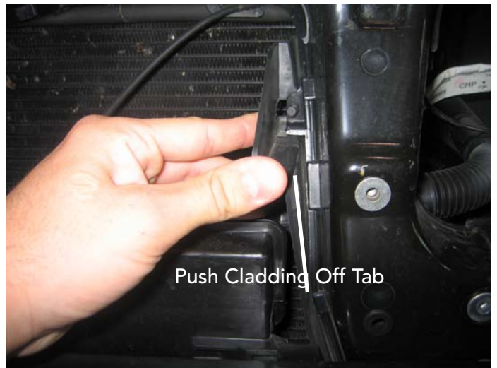
Radiator Cladding Removal
