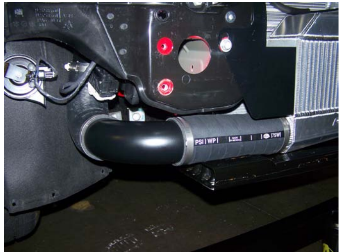
Lower Passenger's Side I/C Tubing Installed (2 Core)
