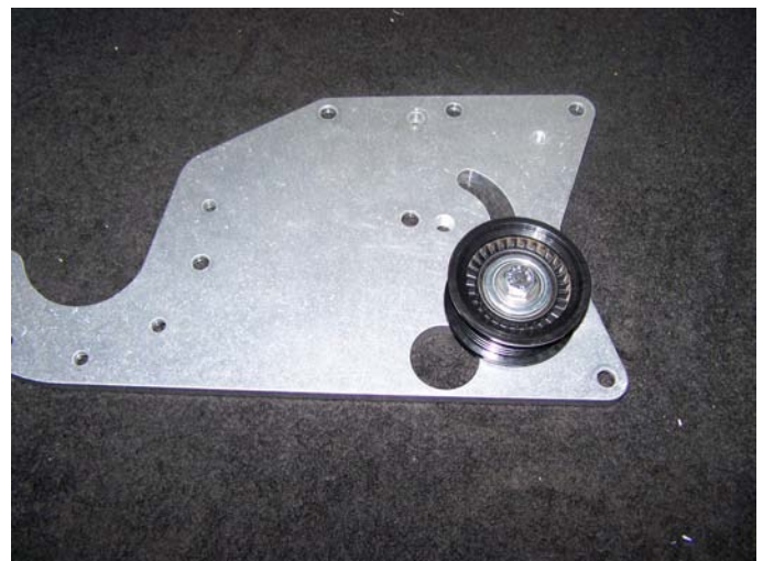
Idler Mounted to Backside of the Bracket
