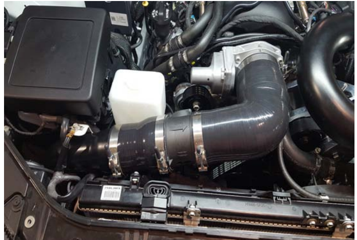
Tubing To Throttlebody Installed
