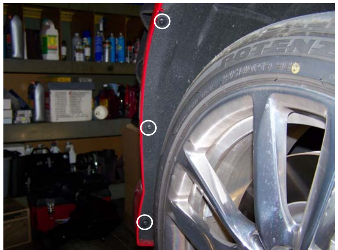
Remove (3) Screws With T-15 Torx Socket
