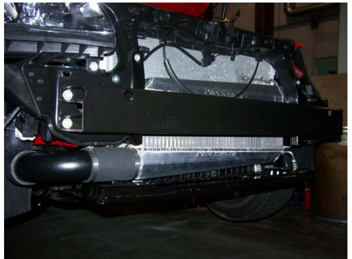
Lower Passenger's Side I/C Tubing Installed (3 Core)
