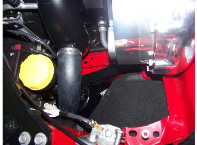
Surge Valve Tube Routing
