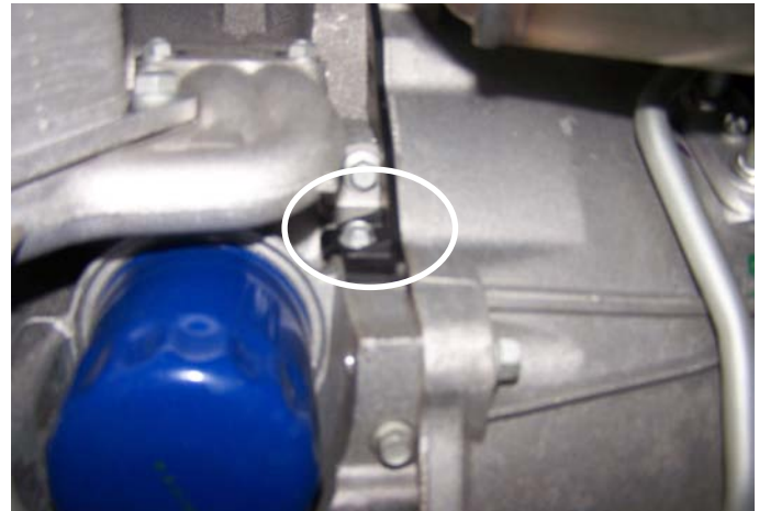
Transmission Access Shield and Hardware
